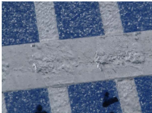
Bottom-view of soldered connection
