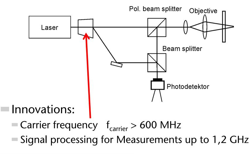
The Ultrahigh Frequency Vibrometer UHF-120 CPolytec
