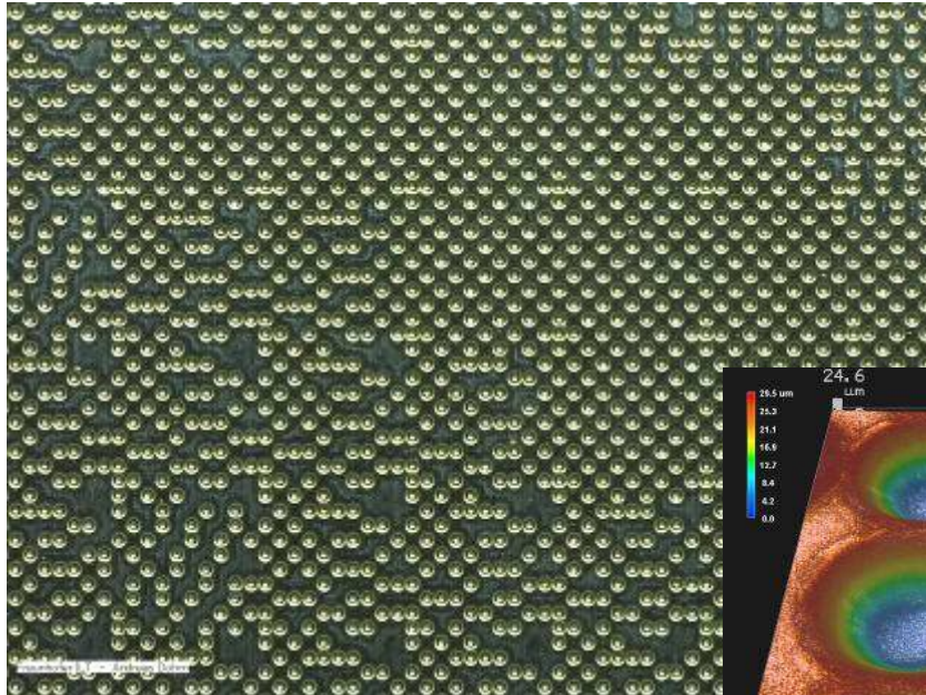
Micro moulding tool for surface structured parts
