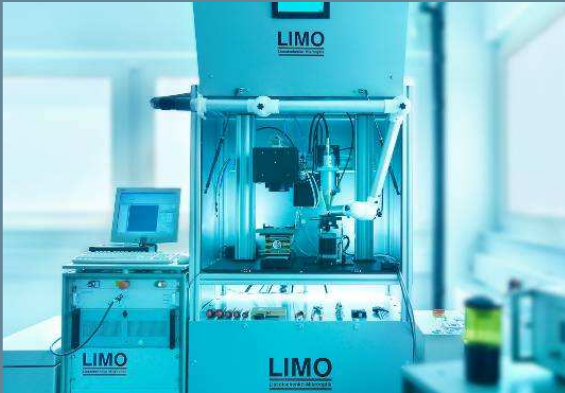
Laser work station with 2D galvo-scanner.
