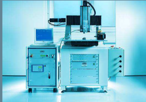
3 axis laser work station with additional rotation axis for cylindrical parts.
