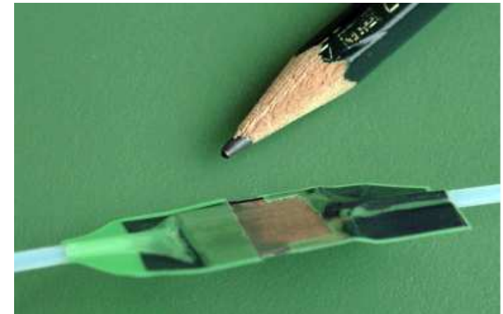
0.5 mm thick fuel cell: photograph (right) and its electrical characteristics
