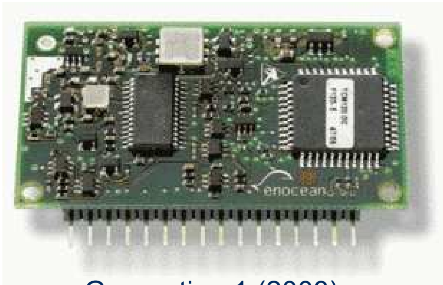
Generation 1 (2003): Discrete components on both PCB sides, 42 x 24 x 5 mm, 5V, 33 mA
