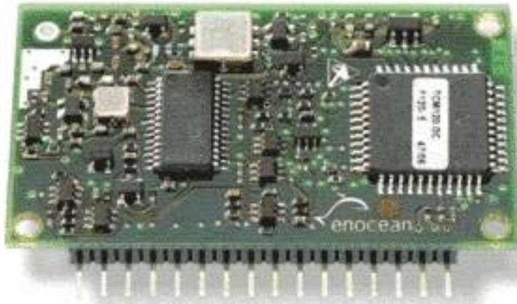
Generation 1 (2004): Discrete components on both PCB sides, 42 x 24 x 5 mm, 5V, 33 mA
